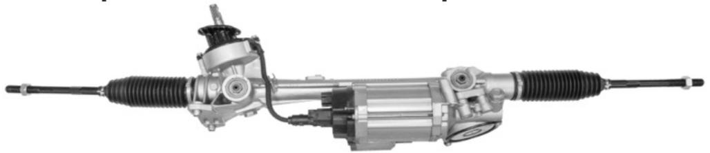
4. With the Power Steering Assist Motor replaced and reconnected, using the same scan tool, perform the SPS function Electronic Power Steering > Programming and follow the on-screen instructions.
