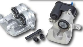
Shaftec knows from its sales data that calipers are subjected to more wear during wintertime. Falling temperatures make the rubber components more brittle and prone to cracking, enabling moisture access and compounding the corrosive issues that are caused by damp and road salt during the winter months.
