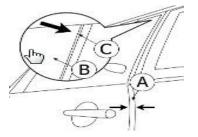
2. Remove the covers A, Loosen the bolts B, Adjust the power window mechanism C, Tighten the bolts B and refit the covers A.
