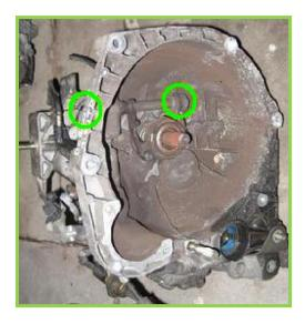
Check the release arm bushes for wear and replace them if necessary to ensure the release arm does not seize. Also the release bearing should be checked for dirt as this may cause it to bind on the shaft.
