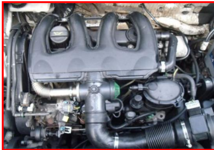
Check the oil filler cap is not loose and pay special attention the engine mounts
