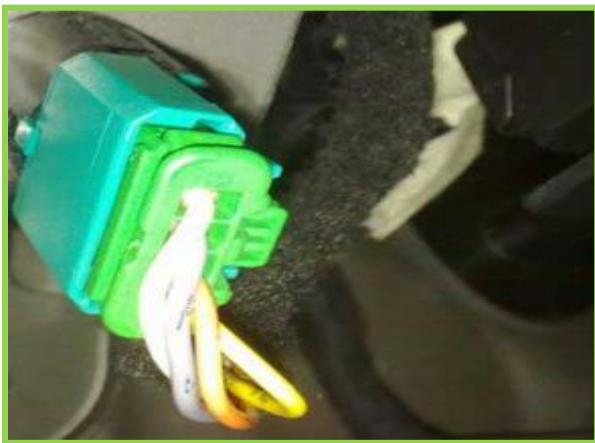
Example of brake light switch and wiring
