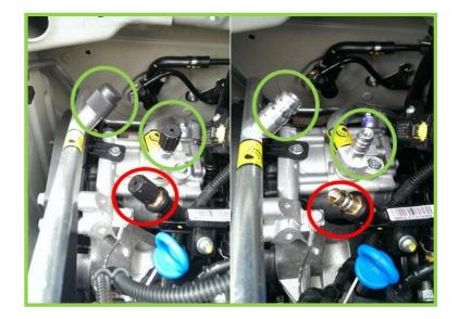
The Valeo Service tech care team have recently seen a number of issues where the air conditioning service machine has been attached to the fuel rail instead of the low pressure port. Petrol has then been extracted into the refrigerant tank. The cost to repair this is very high due to the necessity to have the machine cleaned out and all the internal filters and associated parts replaced.
