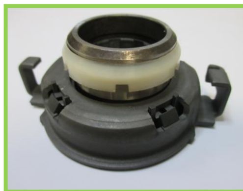
Bearing OK: Guide collar is compressing the circlip allowing smooth entry into the cover
