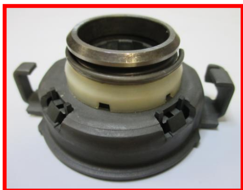
Bearing NOK: Guide collar is not compressing the circlip preventing smooth entry into the cover assembly.
