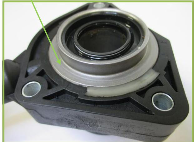
*Apply the gasket compound to the CSC back plate*
