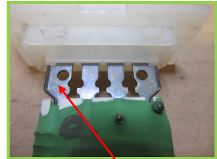
Blueing on the resistors pins
