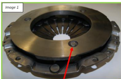
Recessed rivets (below surface area) on pressure plate
