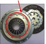
These adaptable kits are designed to replace the original SAT clutch on the vehicle. The original SAT cover has a specific device to maintain the pedal load during the life of the clutch. To compensate, Valeo adaptable kits replacing original SAT kits include discs with low wear facing material.
