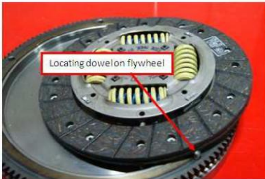
Image showing how clutch plate becomes damaged from locating dowels on flywheel
