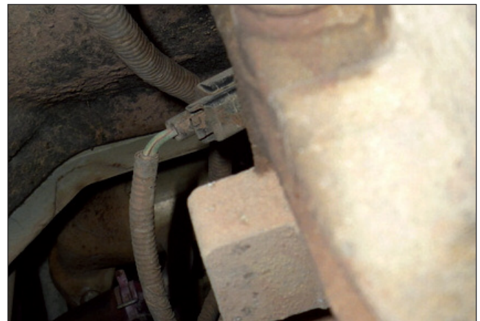
Metal particles can contaminate the timing sensor, so make sure it is clean so that it can work properly.
