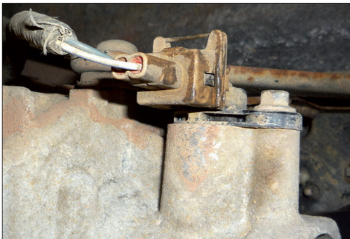
A timing sensor and a road speed sensor are located on the Transit gearbox. The connectors on both sensors can be accidentally switched.
