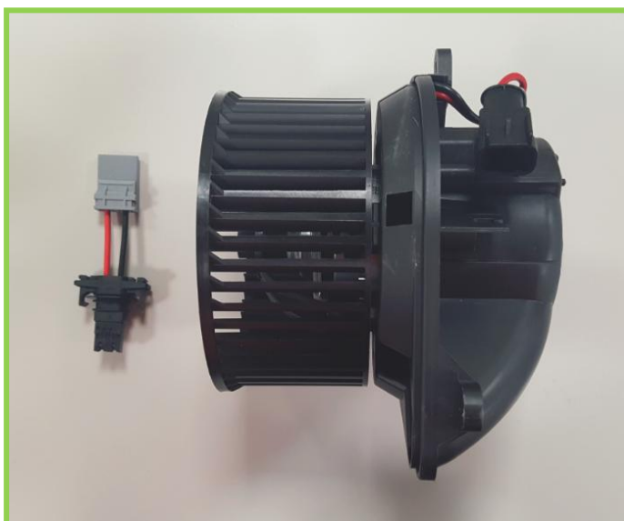
Blower motor 698329 with the additional wiring loom
