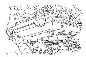
3) Reprogram the faulty on-board network control unit (J519) to ensure compatibility with the new lights.
