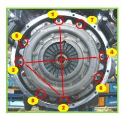
New part taken from Valeo stock; shows no deformation/damage to the straps
