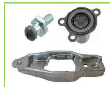
*Figure 3, clutch ball pin, guide tube and release arm
