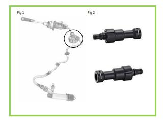
These oscillations/vibrations are experienced by the end user when the clutch pedal is actuated. These symptoms are sometimes incorrectly attributed to a faulty clutch or flywheel but these vibrations can be a result of a faulty/worn or missing frequency modulator (Fig 1 circled) or oscillation absorber (Fig 2).
