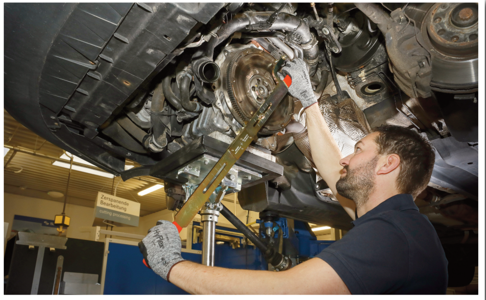
A technician using the ZF tool to assess the condition of the DMF
