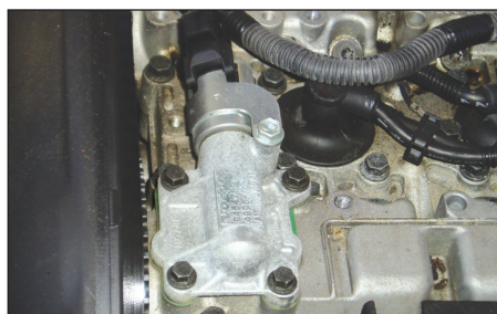
A build-up of oil deposits had intermittently interfered with the variable valve timing
