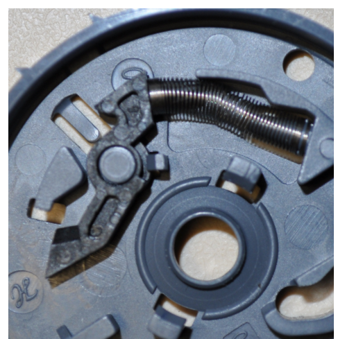
The spring in its proper position
