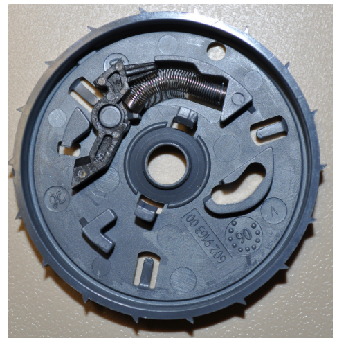
A spring, at top, was unseated, preventing the seat belt reel from releasing the belt
