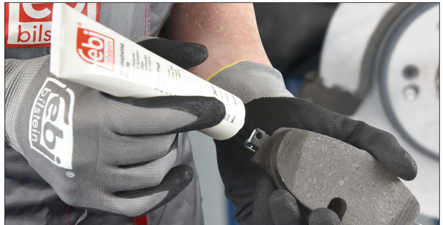
Lubricate the abutment points to ensure free movement and efficient braking by using anti-seize ceramic paste
