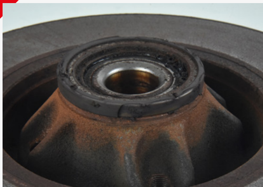
Fig. 1 Damaged reluctor due to contact with the sensor
