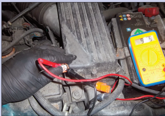
Putting a meter across the ABS connecting cables is the quickest way to test the system.
