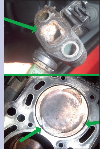
The failed seal on the temperature sender, at top, resulted in damage to the engine block, at bottom.
