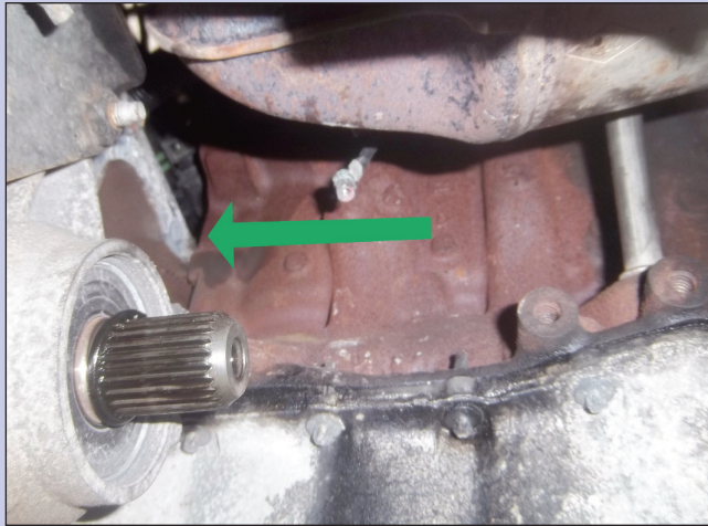
With the driveshaft out of the way, there was plenty of access to remove and refit the starter motor
