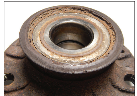
Fig 3. The retractor within the bearing was distorted, cracking the magnetic ring and was the source of the problem
