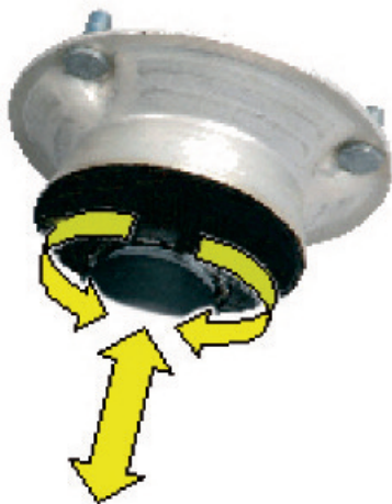
Fig 1. Tension and compression movements have an impact on the strut top mounting
