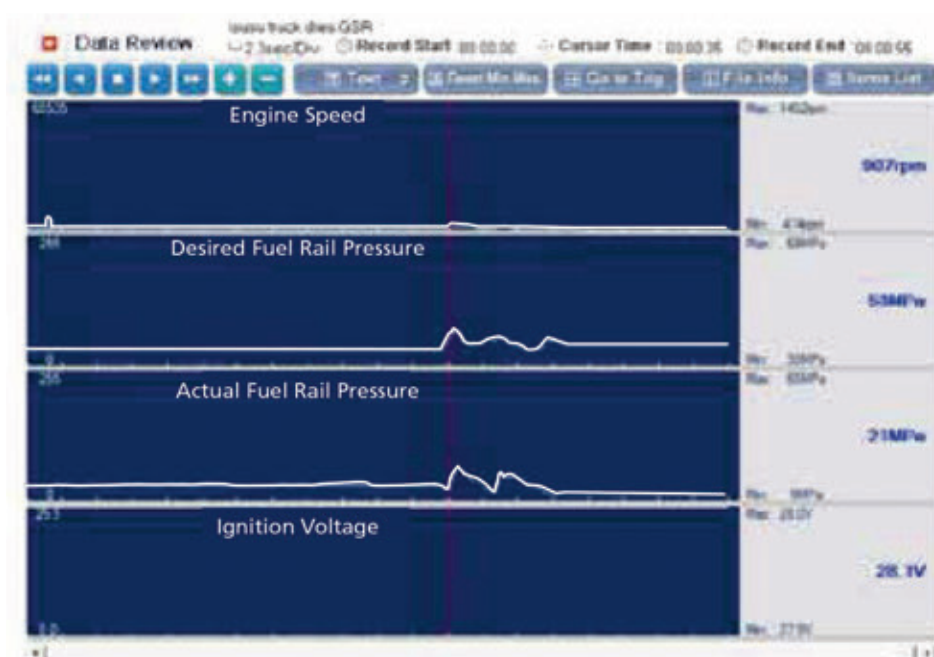
Figure 1 - Discrepancies between desired and actual fuel rail pressures provided the first clue to solving the problem.
