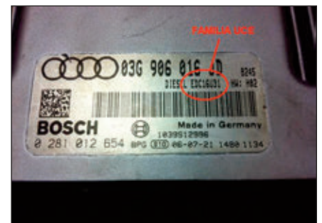
The ECU type can be read off the label
