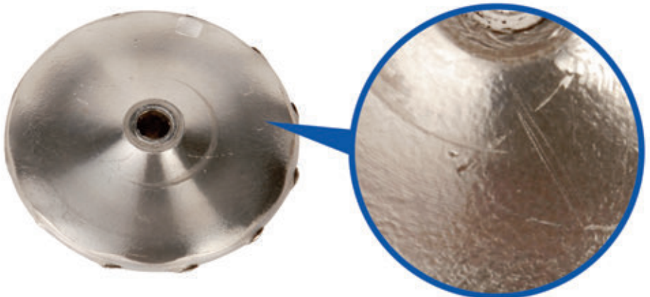
Orange peel on the back of the inducer is another sign of overspeeding
