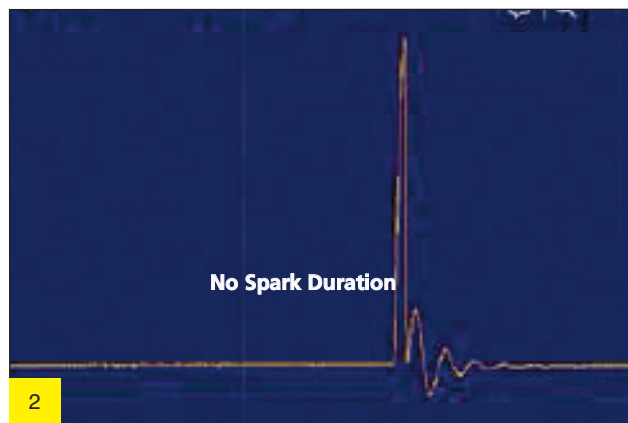
There wasn't any spark duration in cylinder number 4
