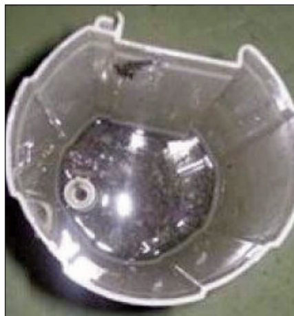
Paint sludge inside the fuel pump assembly
