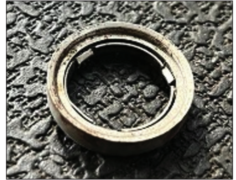
An extra ring was found installed on one of the injectors
