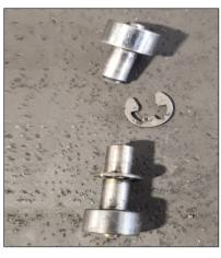
The pin between the motor and the valve had broken
