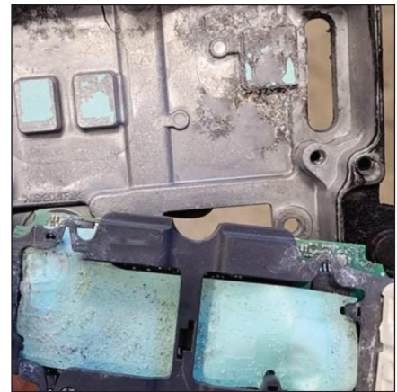
Water had entered into the PTC Heater Module on the Mercedes and had caused a fault
