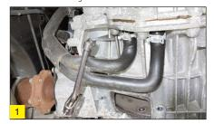
Remove the black plastic blanking cover from the bottom of the bellhousing, this will now give access to the flywheel to drive plate bolts that need to be removed (Fig 2). Remove the three bolts, position a transmission jack under the gearbox to support it's weight and remove the gearbox mounting. Disconnect the propshaft from the rear
