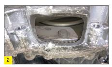
differential by removing the six bolts and remove the centre bearing bracket, which will allow the propshaft to slide away from the differential and hang down.
