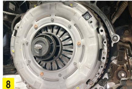
Clean the new clutch pressure plate with clutch and brake dust cleaner, to ensure the face is degreased and, using a clutch alignment tool, mount the new clutch (Fig 8). Tighten the bolts in an even and sequential manner and then torque to the
