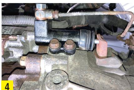
pipe bracket bolt. Ease the slave cylinder away from the gearbox, and remove the air charge cooler pipe that runs under the engine/gearbox. Detach the lower gearbox pendulum mounting and retaining bracket, as well as the tin cover plate at the bottom of the bellhousing. Remove the lower bellhousing bolts, leaving a couple of easily accessible bolts to support the gearbox until the point of removal, lower the lift to waist height and
