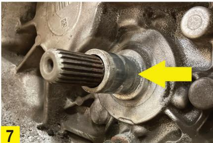
Remove the release bearing from the gearbox and clean the bellhousing area with clutch and brake dust cleaner, and check the bearing guide tube for wear (Fig 7) as it is known for both Hyundai and Kia engines to wear in this area and cause release problems.
