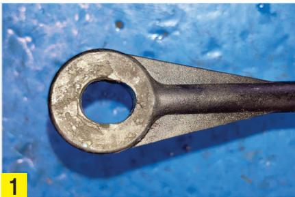
The clutch master cylinder was replaced, the clutch bled and full clutch pedal travel restored, but gear selection with the engine running was still difficult. However, with the engine switched off, the gears could be selected easily, which indicated that the clutch was not fully disengaging. Authorisation was given to remove the gearbox for further investigation.
