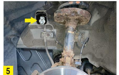
remove the two gearbox mounting bolts that are accessed through the inner wing (Fig 5), then lower the lift and remove the mounting from the gearbox. Raise the lift to gain access to the underside, support the gearbox with a transmission jack and remove the final bellhousing bolts. Ease the gearbox away from the engine. When the gearbox input shaft is clear of the clutch, lower the gearbox, remove the gearbox from the vehicle and place it somewhere safe.
