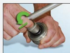
The tool jams immediately and cannot be turned when moved in an anti-clockwise direction.
