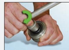
**The tool can be continuously turned in a clockwise direction with slight resistance**
