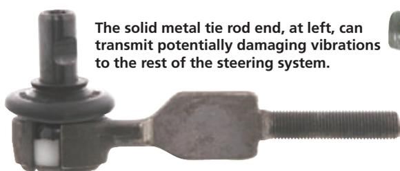
**The solid metal tie rod end, at left, can transmit potentially damaging vibrations to the rest of the steering system.**
