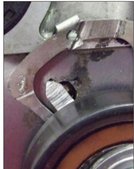
The upside down tensioner left no clearance room for the timing belt, as can be seen by the scoring in this picture
