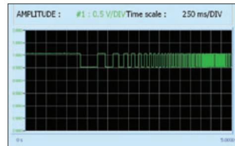
Figure 3: Oscilloscope trace of the signal voltage of the wheel speed sensor as the wheel accelerates from a stop position
