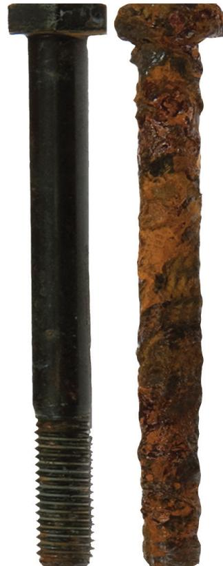
**Meyle's zinc-nickel coated VAG replacement suspension bolt, at left, after a 480 hour salt spray endurance test. The other bolt is an OE suspension bolt, after the same test.**
