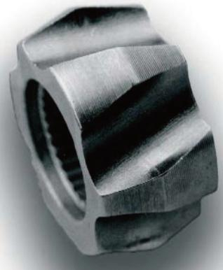
Examine the hub inside the CV joint for any wear, beyond polishing
