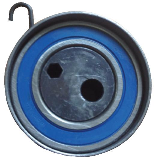
**The newer design, spring loaded timing belt tensioner for Opel evergreen 1.7l diesel engines**
