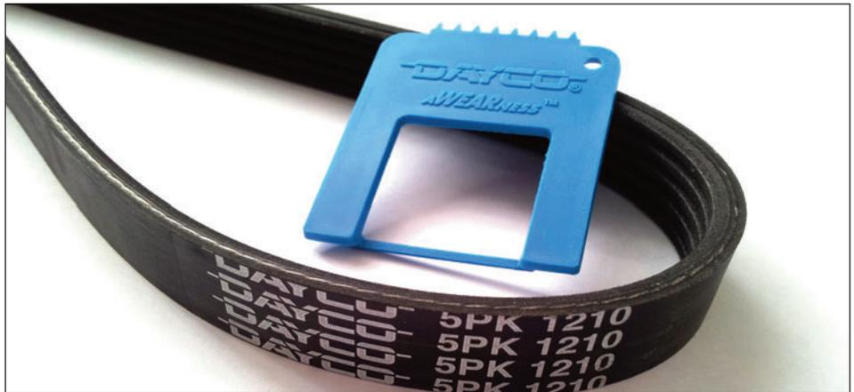
As a result, the 'V' profiles of the ribs on the belt begin to wear down and start to resemble a 'U' and not a 'V'. As the profile changes, the contact area of the belt on the pulley is reduced, and the efficiency of the belt drops. This wear can lead to slippage and affect the performance of the belt, as well as make it very noisy.
