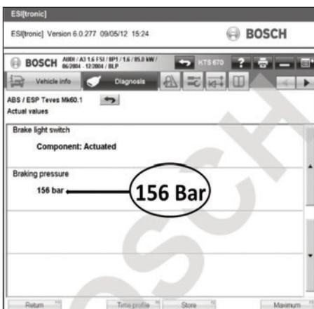
Any brake application will change the status of the brake light switch and will raise the braking pressure accordingly
