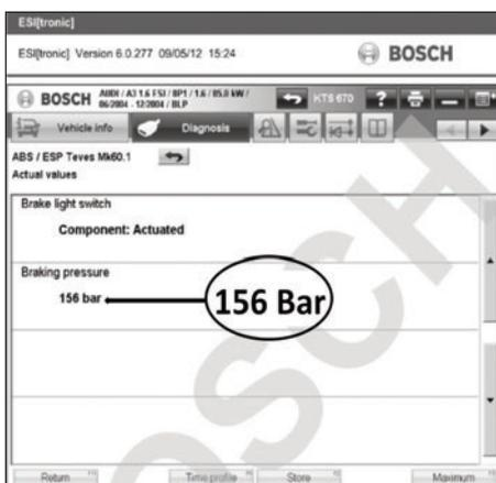
**Any brake application will change the status of the brake light switch and will raise the braking pressure accordingly**
