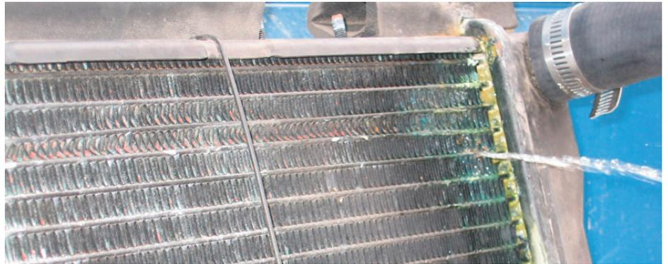
itself. This type of electrolysis is a chemical reaction between the coolant and the aluminium, that is basically like a battery. When the coolant is "worn out", it acts like acid in a battery, allowing dissimilar metals to create voltage and a current. The cure for this type of electrolysis is simple: replace the damaged parts, flush the cooling system and refill with the proper coolant.
