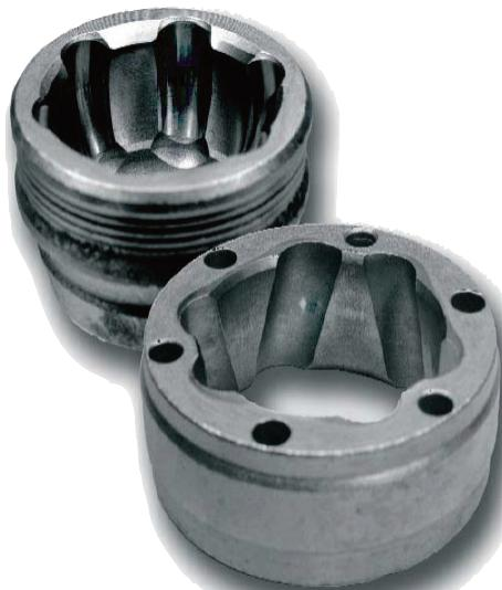
Examine the interior of the CV joint for any wear, beyond polishing
