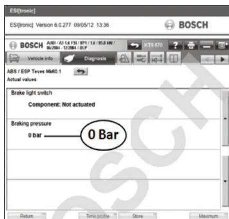
**Without brakes applied, the brake pressure is zero and the brake light switch is not actuated**
