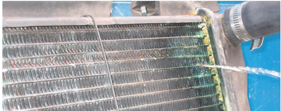
itself. This type of electrolysis is a chemical reaction between the coolant and the aluminium, that is basically like a battery. When the coolant is "worn out", it acts like acid in a battery, allowing dissimilar metals to create voltage and a current. The cure for this type of electrolysis is simple: replace the damaged parts, flush the cooling system and refill with the proper coolant.
