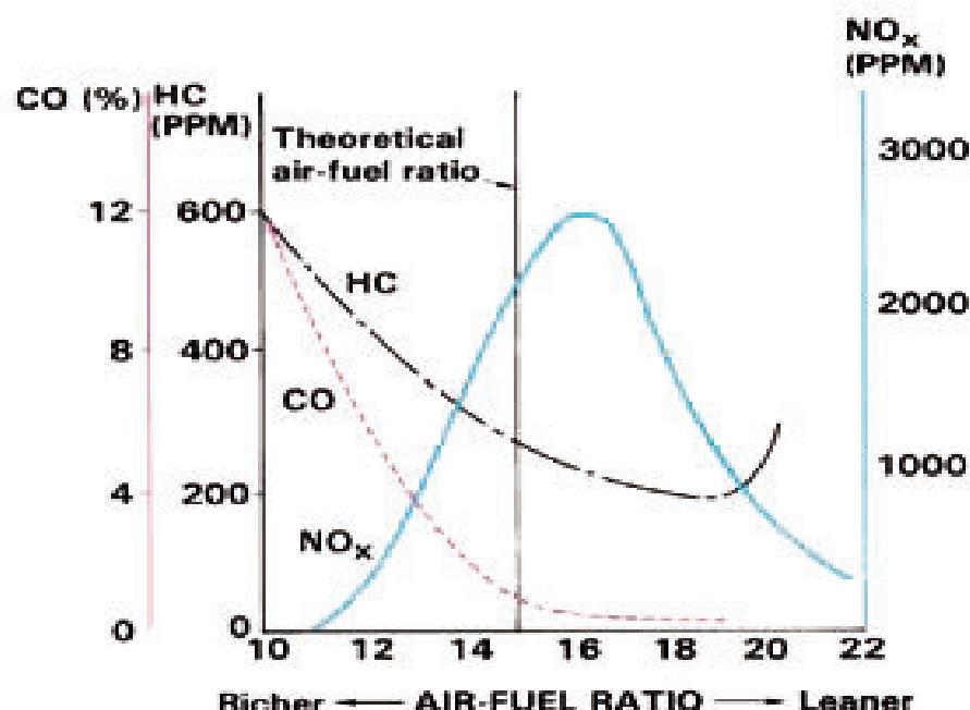
Figure 2 The effect of air-fuel ratio and CO (red line), HC (black line) and NOx (blue line)
