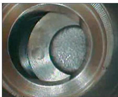
Valves can be examined by inserting the probe in the spark/glow plug hole
