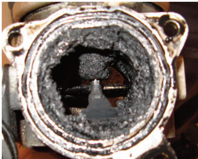
This car was running poorly. The accumulated sludge, varnish and soot obviously would be causing problems.
