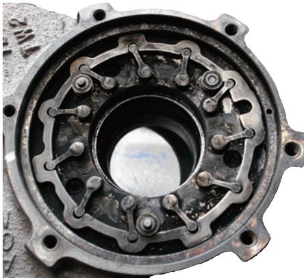
**A view of the ring that controls the position of the vanes, which change the boost provided by the turbo**
