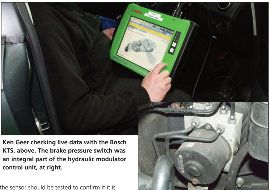
Ken Geer checking live data with the Bosch KTS, above. The brake pressure switch was an integral part of the hydraulic modulator control unit, at right.
