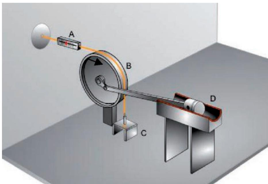
**A simplified version of a dynamometer testing an engine. This simple arrangement can determine the torque and power of the engine being tested.**
