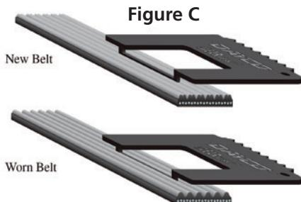
**A new or serviceable belt, on top, and a worn belt that needs replacement, on bottom.**
