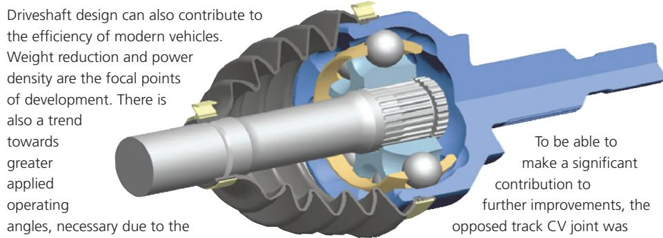
To be able to make a significant contribution to further improvements, the opposed track CV joint was developed as the alternative to the Rzeppa joint.
