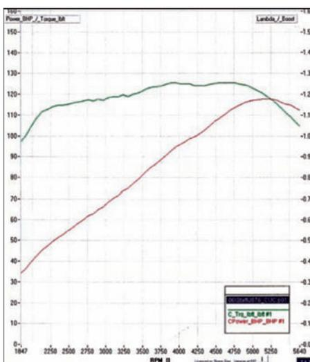
**A typical torque/power graph for a mid-performance, naturally aspirated, petrol engine**
