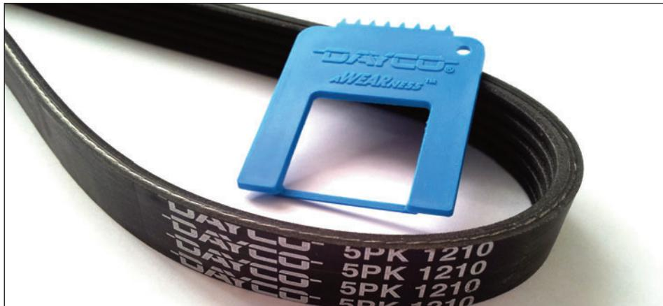
As a result, the 'V' profiles of the ribs on the belt begin to wear down and start to resemble a 'U' and not a 'V'. As the profile changes, the contact area of the belt on the pulley is reduced, and the efficiency of the belt drops. This wear can lead to slippage and affect the performance of the belt, as well as make it very noisy.
