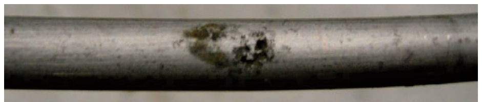
A pin-hole leak on a fuel line was sucking air into the line, but wasn't leaking diesel yet
