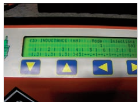
Measured inductance of each injector, note the obvious fault in No. 4
