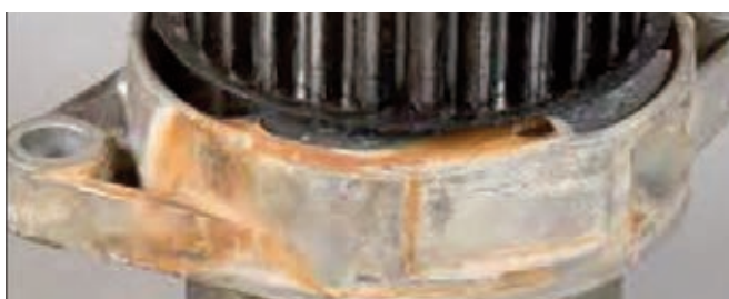
Cooling problems can arise from any part of the system, like this leaking water pump
