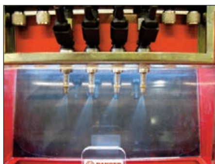
The ASNU test bench shows the performance of each injector
