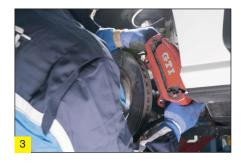
Tighten the driveshaft bolt by hand before refitting the wheel, with its bolts also secured hand tight, and lower the vehicle to the floor to tighten the driveshaft bolt. Please note, that if the underside of the bolt is not smooth the torque value is 70Nm plus 90, whereas if its underside is smooth, the value is 200Nm plus 180.
