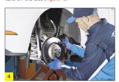
Remove the metal cap that protects the axle shaft bolt and, without the use of an impact wrench, unscrew it and then take off the wheel bearing.
