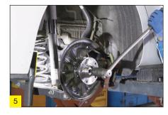
Reposition the brake disc and secure the screws to 8Nm, followed by the brake caliper, torqueing its bolts to 90Nm plus 90, before refitting the wheel and tightening the wheel bolts to 120Nm.
