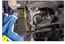
Clean the bearing housing and remove any oxidation, then lubricate the cleaned surface, but before installing the new wheel bearing (Dayco part number KWD1021), check that the magnetic sensor ring is intact through the indication bars on Dayco Tool 19 (Figure 2).
